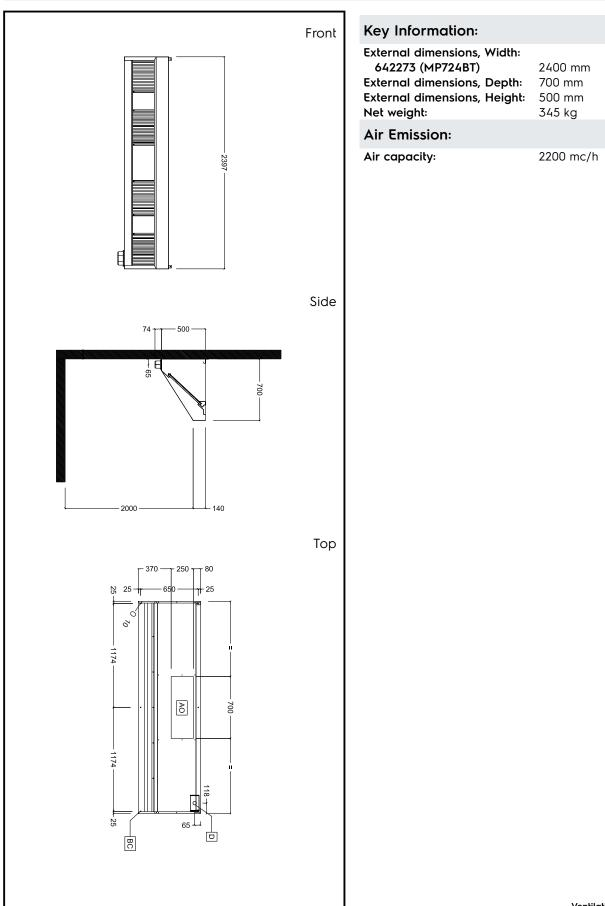
Ventilation Equipment 430 S/S Wall Hood+Filters 2400X700mm
